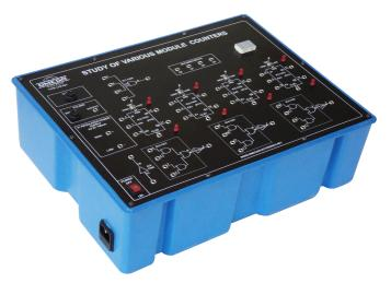
**OMEGA TYPE LTB-823** Computer Logic Training Board has been designed specifically to study Various Module Counters. This Training Board gives a better understanding of the design, working & practical aspects of counters. Gates and flip-flops can be used to construct any type of counter. Output of each counter circuit can also be observed in decimal code with the help of the seven segment displays. The board is absolutely self contained and requires no other apparatus.
