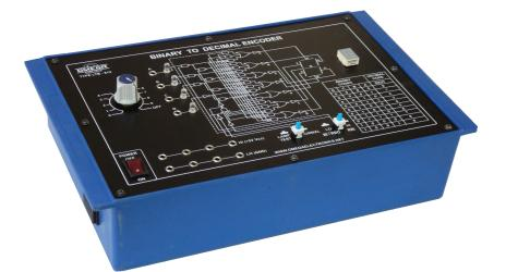
OMEGA TYPE LTB-814 Computer Logic Training Board has been designed specifically for the study of Binary to Decimal Encoder. There are arrangements for changing the binary input with the help of a selector switch as well as to feed the unknown 4-bit binary code to read decimal value on seven segment display. The board is absolutely self contained and requires no other apparatus.
