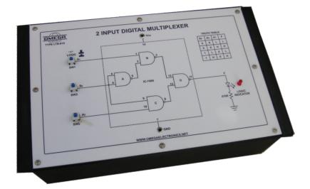
**OMEGATYPE LTB-815** Computer Logic Training Board has been designed specifically for the study of 2-Input Digital Multiplexer. The technique of multiplexing is frequently used where a number of digital signals are to be processed simultaneously or sent together over a significant distance to minimizes the number of circuits or communication channels. The board is absolutely self contained and requires no other apparatus.
