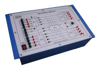
OMEGA TYPE LTB-832 Computer Logic Training Board has been designed specifically for the study of Bilateral Switch. This Training Board gives a better understanding of two way communication interface between data buses. The board is absolutely self contained and requires no other apparatus.
