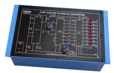
OMEGA TYPE LTB-833 Computer Logic Training Board has been designed specifically for the Study of 8-Bit Analog to Digital Converter. This Training Board gives a deep understanding of the conversion of Analog signal into Digital signal using ICADC 0800, which is based on Successive approximation method of Conversion. Practical experience on this board carries great educative value for Science and Engineering Students.
