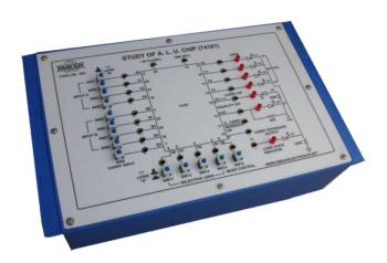
OMEGA TYPE LTB-824 Computer Logic Training Board has been designed specifically for the study of Arithmetic & Logic function by using 74181 chip. The board is absolutely self contained and requires no other apparatus.
