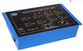
OMEGA TYPE LTB-826 Computer Logic Training Board on Flip-Flops has been specifically designed to give students an idea about Flip-Flops and to study different types of Flip-Flops. The output of the Flip-Flops can be observed with the help of logic level indicators (LEDs), which are provided on the panel. The board is absolutely self contained and requires no other apparatus.
