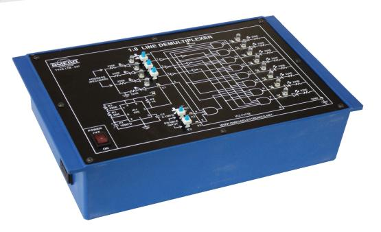
**OMEGA TYPE LTB-837** Computer Logic Training Board has been designed specifically for the study of 1:8 Line Demultiplexer. This Training Board gives a better understanding of the phenomena of demultiplexing with one input demultiplexed to eight outputs using three control inputs (Address).
