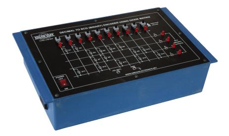
OMEGA TYPE LTB-854 Computer Logic Training Board has been designed specifically for the study of Decimal to BCD Encoder using Diode Matrix. This Training Board gives a better understanding of the phenomenon of encoding with decimal input and BCD (binary coded) output using diodes.
