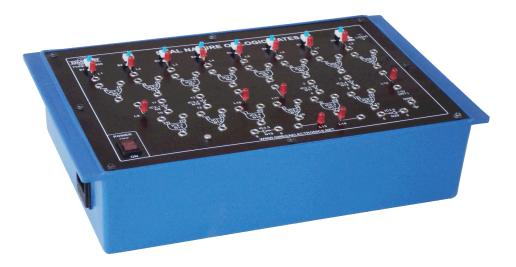
**OMEGA TYPE LTB-859** Computer Logic Training Board has been designed specifically for the study of Dual Nature of Logic Gates. This Training Board gives a better understanding of the phenomena of duality with the help of verification of truth tables of Dual gates. This board also explains combinational logic function Boolean variables and generation of truth tables.
