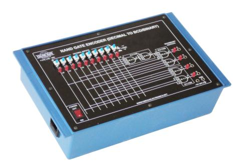
OMEGA TYPE LTB -856 Computer Logic Training Board has been designed specifically for the study of NAND gate Encoder, to encode Decimal number to BCD(binary coded) equivalent. This Training Board gives a better understanding of the phenomena of encoder using four input NAND gates with ten decimal inputs and 4-bit binary output.
