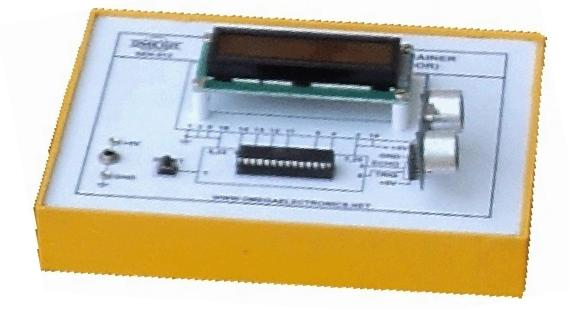
OMEGA TYPE ICT-911 Experimental Set Up has been designed specifically for determining the soil distance of any object or obstacle using Ultrasonic Sensor by the application of ultrasonic waves. The LCD panel directly displays measured distance.
