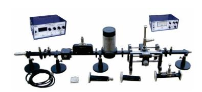
OMEGA TYPE ES-501 uses low power reflex klystron along with its klystron power supply and klystron mount, as a microwave signal source along with other standard high quality components and VSWR meter, enables to perform under mentioned experiments in the laboratory. The waveguide components are based on rectangular waveguide equipped with rectangular plain flanges.
