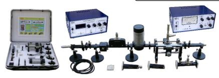
**OMEGA TYPE ES-502** uses Gun oscillator with its Gun power supply and Pin modulator as a microwave signal source along with other standard high quality components and VSWR meter, enables to perform under mentioned experiments in the laboratory. The waveguide components are based on rectangular waveguide equipped with rectangular flange.
