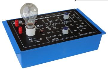
**OMEGA TYPE PET-404** Power Electronic Training Board has been designed specifically to study the characteristics of a TRIAC and its application as A.C. Power Control using phase control technique. The unit is provided with built-in load facility. Experiments for the study of radio frequency interference in phase control and methods of their suppression, can be conducted on this training board.
