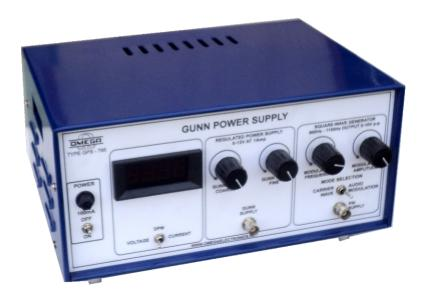
**OMEGA TYPE GPS-795** Designed to protect Gunn diode from reverse voltage application, over voltage and transient low frequency oscillations. Gunn Power Supply comprises of an electronically regulated DC power supply and a square wave generator, designed to operate Gunn-Oscillator and Pin Modulator simultaneously. The front-panel meter monitors the Gunn voltage and the current drawn by the Gunn-diode.
