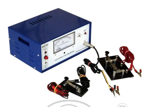
**OMEGA TYPE ECM - 110** Electronic Coulomb-meter is suitable for charge measurement in the range of 10nC to 10uC. It uses a large 4½" x 2½" rectangular meter for easy reading. For good many experiments it replaces conventional Ballistic Galvanometer. While using Ballistic Galvanometer, much of the time, care and thought of the students goes to it, so that the actual measurement becomes secondary.
