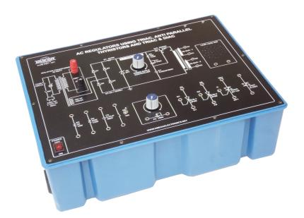
OMEGA TYPE PET-421 Power Electronic Training Board has been designed specifically for to study A.C. Regulators using triac, antiparallel thyristor and triac & diac.
