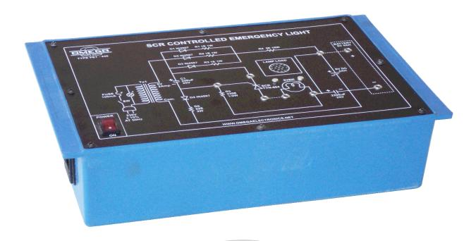
**OMEGA TYPE PET-438** Power Electronic Training Board has been designed specifically for the study of SCR Controlled Emergency Light. The board is absolutely self contained and requires no other apparatus.
