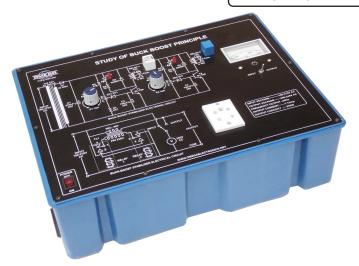
**OMEGA TYPE PET-451** Study of buck boost principle has been designed with a view to provide practical/experimental knowledge of Automatic two step Buck Boost Principle with electronically controlled circuit.
