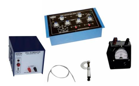
**OMEGA TYPE ES-203** Experimental Set Up has been designed specifically to determine the specific resistance of the material of a wire using P.O. Box. The set up is absolutely self contained and requires no other apparatus.
