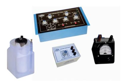
**OMEGA TYPE ES-204** Experimental Set-up has been designed specifically to determine the internal resistance of a primary cell (Leclanche Cell) by Mance's method using P.O. Box. The set up is absolutely self contained and requires no other apparatus.
