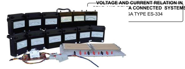
OMEGA TYPE ES-334 Experimental setup has been designed specifically to verify the voltage and current relations in star and delta connected systems.
