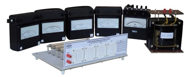
OMEGA TYPE ES-335 Experimental setup has been designed specifically to calculate phasor sum of current in an ac circuit is zero. The setup is complete in all respect and requires no other apparatus.
