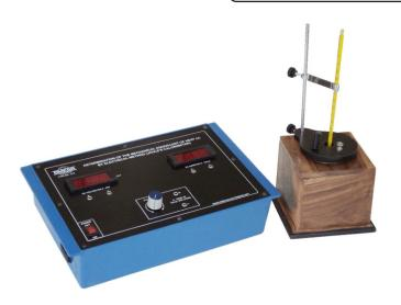
**OMEGATYPE ES-213** Experimental Set Up has been designed specifically to determine the mechanical equivalent of Heat (J) by electrical method (Joule's Calorimeter).
