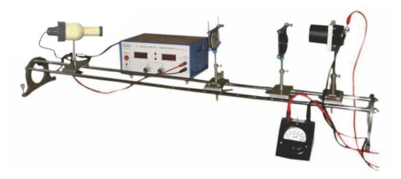
**OMEGA TYPE ES-214** Experimental Set Up has been designed specifically for the determination of PLANCK'S CONSTANT using SOLAR CELL. (PHOTO VOLTAIC CELL) and three optical filters with the help of Wien's Radiation Law and to study inverse square law.
