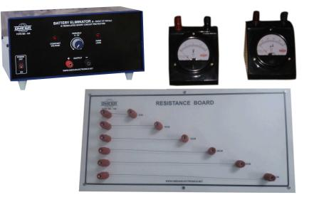
**OMEGA TYPE ES-217** Experimental Set Up has been designed specifically to determine the relationship between the resistance and length of wire using an ammeter and a voltmeter.
