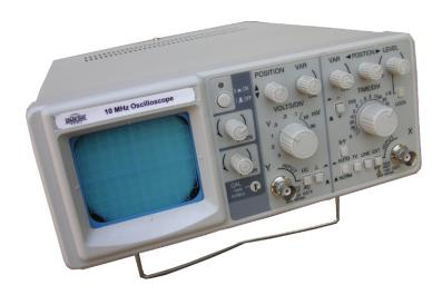
**OMEGA TYPE CRO-10** This Oscilloscope is corresponding to horizontal style with small size. The bandwidth of Y axis is DC $\sim$ 10MHz and the deflection factor is 5mV $\sim$ 5V/DIV. It can be up to 50V/DIV supplying with the 10.1 probe. Sweep deflection factor is 0.1us/div-0.1s/div. It has the Following features wide measurement, high sensitivity trigger lock and etc. Sweep switch adopt code switch and accuracy orientation. It is convenient to operate.
