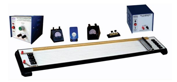
**OMEGATYPE ES-208** Experimental Set Up has been designed specifically to calibrate a Voltmeter with the help of Potentiometer. The set up is absolutely self contained and requires no other apparatus.
