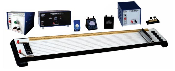
OMEGA TYPE ES-209 Experimental Set Up has been designed specifically to calibrate an ammeter with the help of a Potentiometer. The set up is absolutely self contained and requires no other apparatus.
