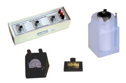
**OMEGA TYPE ES-224** Experimental Set Up has been designed specifically to determine internal resistance of a cell (Leclanche cell) using a voltmeter and resistance box. The set up is absolutely self contained and requires no other apparatus.
