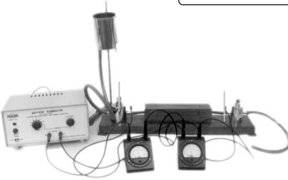
OMEGATYPE ES-227 Experimental Set Up has been designed specifically To determine Mechanical equivalent of heat by "J" Callendar and Barne's method
