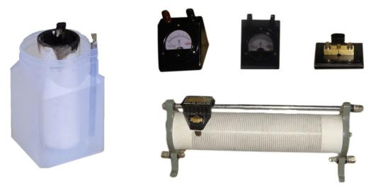
**OMEGA TYPE ES-220** Experimental Set Up has been designed specifically to determine the internal resistance of a cell using an ammeter and a voltmeter. The set up is absolutely self contained and requires no other apparatus.
