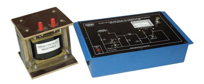
**OMEGA TYPE ES-221** Experimental Set Up has been designed specifically for the study of rise and decay of current in an LR circuit with source of constant EMF. We use an Inductor (of high inductance and low resistance) in order to enable one to make measurements of the rise and decay current.
