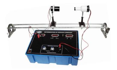
**OMEGATYPE ES-230** Experimental Set Up has been designed specifically for determination of Stefan's constant by using an incandescent Lamp and Photo Voltaic Cell. It is based on Stefan-Boltmann relation. The set up is absolutely self contained and requires no other apparatus.
