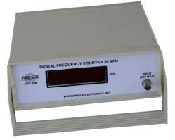
**OMEGA TYPE DFC-20M** Digital Frequency Counter is a simple to operate but accurate and reliable test equipment. The circuit is based on micro-controller.
