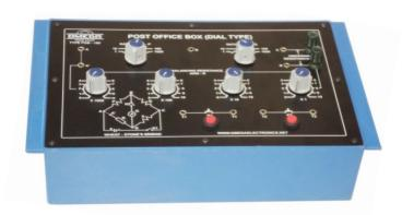
**OMEGA TYPE POB-180** Dial Type Post Office Box is a precision instrument intended for general laboratory use. In this POB-180, the resistance are arranged such that these can be grouped into three branches which forms the three arms of a Wheatstone's Bridge, the fourth arm can be formed by connecting the unknown resistance across the terminals marked "UNKNOWN". The basic Wheat Stone's Bridge circuit is also shown on the panel for easy understanding.
