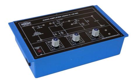
**OMEGA TYPE ETB-247** Experimental Training Board has been designed specifically for the study of Audio Amplifier using LM-380.
