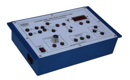
**OMEGA TYPE ETB-248** Experimental Training Board has been designed specifically to study the Logarithmic Amplifiers Design & Test (using-741 Op-Amp.)
