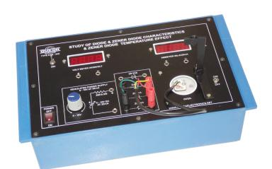
**OMEGA TYPE ETB-245** Experimental Training Board has been designed specifically for plotting the forward and reverse bias characteristics of a Germanium semiconductor Diode and Zener Diode and study of temperature coefficient of Zener Diode. The board is absolutely self contained and requires no other apparatus.
