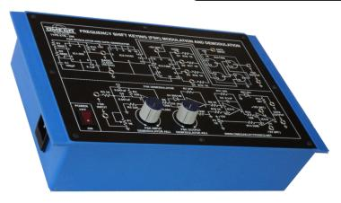
**OMEGA TYPE ETB-206** Experimental Training Board has been designed specifically for the study of frequency shift keying modulation and demodulation.
