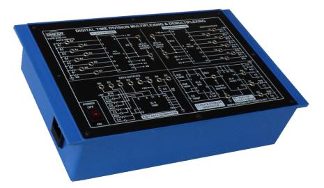
**OMEGA TYPE ETB-211** Experimental Training Board has been designed specifically to study Digital time division multiplexing & demultiplexing. 8 channel Digital Multiplexer and Demultiplexer are provided on the Trainer. A rolling Address Generator scans the 8 channels sequentially. Data Generator with 8 different outputs act as signal sources for the 8 channels.
