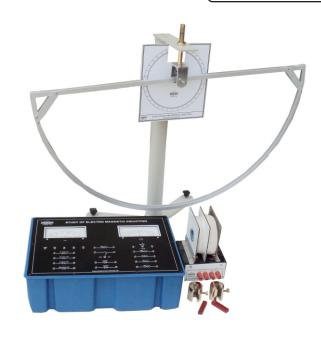
**OMEGATYPE ES-232** Experimental Set Up has been designed specifically for the study of electromagnetic induction and verification of Faraday's law. The set up is absolutely self contained and requires no other apparatus.
