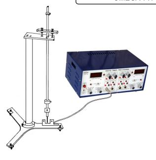
**OMEGATYPE ES-234** Experimental Set Up has been designed specifically to study the viscous fluid (air) damping of a compound pendulum. It also aims at determining the damping co-efficient and Q of the oscillator. The set up is absolutely self contained and requires no other apparatus.
