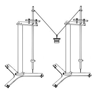
**OMEGATYPE ES-237** Experimental Set Up has been designed specifically for the study of coupled pendulum system, study of oscillations in mixed modes & determination of the period of energy exchange between the two oscillators. The set up is absolutely self contained and requires no other apparatus.
