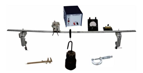
**OMEGA TYPE ES-243** Experimental Set Up has been designed specifically determination the young's modulus by bending of beam / flexure & lever method. A Galvanometer and Cell Eliminator may be used for determining the exact contact setting.
