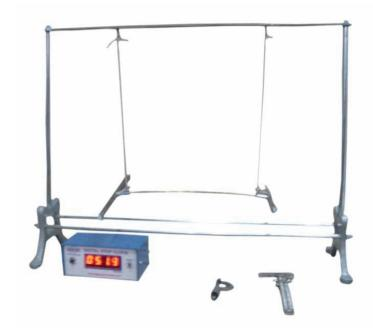
OMEGA TYPE ES-244 Experimental Set Up has been designed specifically to find the value of Young's modulus (Y), modulus of rigidity (n) and Poisson's ratio (s) by Searle's Apparatus.
