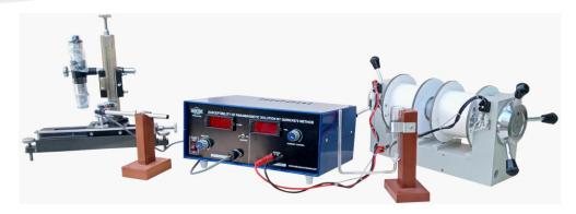
**OMEGA TYPE ES-247** Experimental Set Up has been designed specifically for the Measurement of magnetic susceptibility of paramagnetic solution by Quincke's method. Also find the ionic molecular susceptibility of the ion and magnetic moment of the ion in terms of Bohr magnetron. The set-up consists of Electromagnet, Constant Current Power supply (0 - 4Amp), Digital Gauss meter with Hall probe, Traveling microscope, Quincke's tube with stand, sample (FeCI3).
