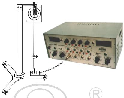
**OMEGATYPE ES-238** Experimental Set Up has been designed specifically to study the variation of time period with amplitude in large angle oscillations using Compound Pendulum. The set up is absolutely self contained and requires no other apparatus.
