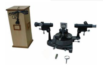
**OMEGA TYPE ES-252** Experimental Set Up has been designed specifically for the Measurement of Wavelength of prominent lines of mercury by Diffraction Grating Method. The set-up consists of Spectrometer, Diffraction Grating, Mercury light source, Reading lens etc.
